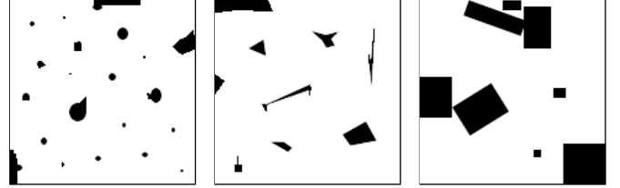
Fig. 4. 2D obstacle maps of the evaluated scenarios. Each map covers an area of 1.5 \text{ m} \times 1.5 \text{ m} at 0.01 \text{ m} resolution. Planar obstacles are marked in black.
